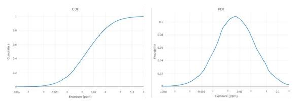
d. The percentile values for the expected exposure are displayed under the "Exposure Estimates" tab. In the case study displayed here, using the model we parameterized, we expect the median exposure for the population to be approximately 0.0069ppm.
